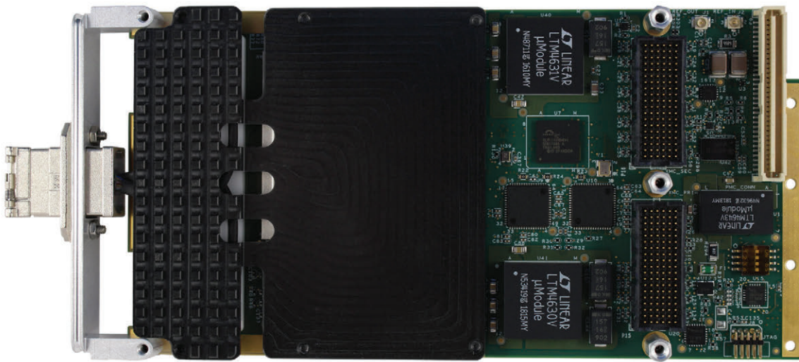
Figure 1: The V1153 is a rugged XMC FPGA card for high-speed interface and coprocessing solutions. It offers 4 to 12 optical port options (front panel or backplane) as well as 1-16Gbps electrical backplane ports.
